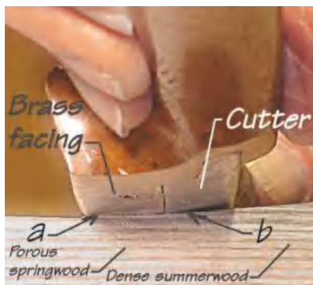
▲ Pic.3 Here the 'shave cuts almost parallel to the grain
